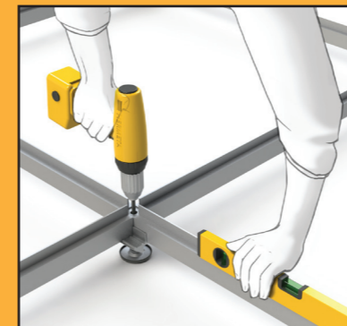
adjusting the floor
